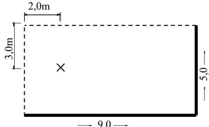
✗ ... Position of the desired suspension point
